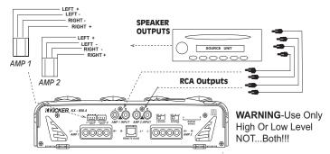
The use of twisted pair interconnects is recommended for all installations to minimize noise. When routing these cables through the automobile, try to keep them away from factory wiring harnesses and other power wiring. If you need to cross any of this wiring do so at a 90 degree angle to reduce the potential of noise problems.
